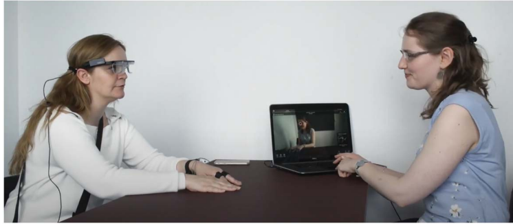
Figure 1. Picture of the experimental setting. (Left) A participant wearing eye-tracking glasses and electrodermal activity sensors. (Right) The experimenter setting up the eye-tracking glasses software.
